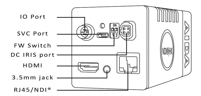
2. Test the video either through HDMI or NDI. The camera will be default resolution of 1080 30p.
